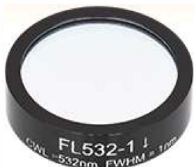
FL532-1 Ø1" Filter CLW = 532 nm, FWHM = 1 nm
