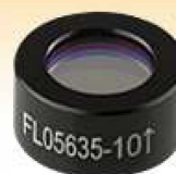
FL05635-10 Ø1/2" Filter CWL = 635 nm, FWHM = 10 nm
